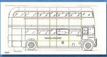
General Arrangement drawing highlighting the tooling adjustments on the RML casting.
