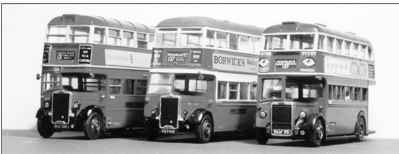
London Transport Leyland STD family The three varieties of STD as would have been seen about 1949. From the left: 1937 TD4 (Little Bus Company kit), 1941 TD7 (scratchbuilt) and 1947 PD1 (modified EFE diecast). Construction and modification by Rod Blackburn.
